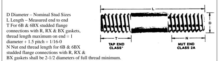
Tap End Studs are available in ASTM A193 Grades of material or special materials. Sigma stocks the most frequently used sizes of tap end studs in ASTM A193 Grade B7. Tap end studs can also be plated or coated if allowances are made for coating thickness and thread fit.
